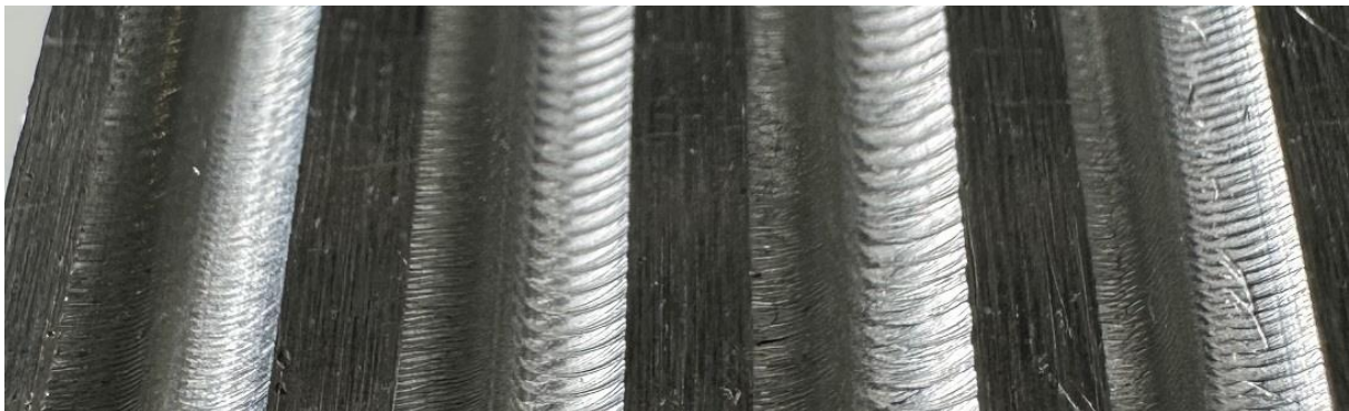
Figure 4.4 Surface of the workpiece with chatter marks.
