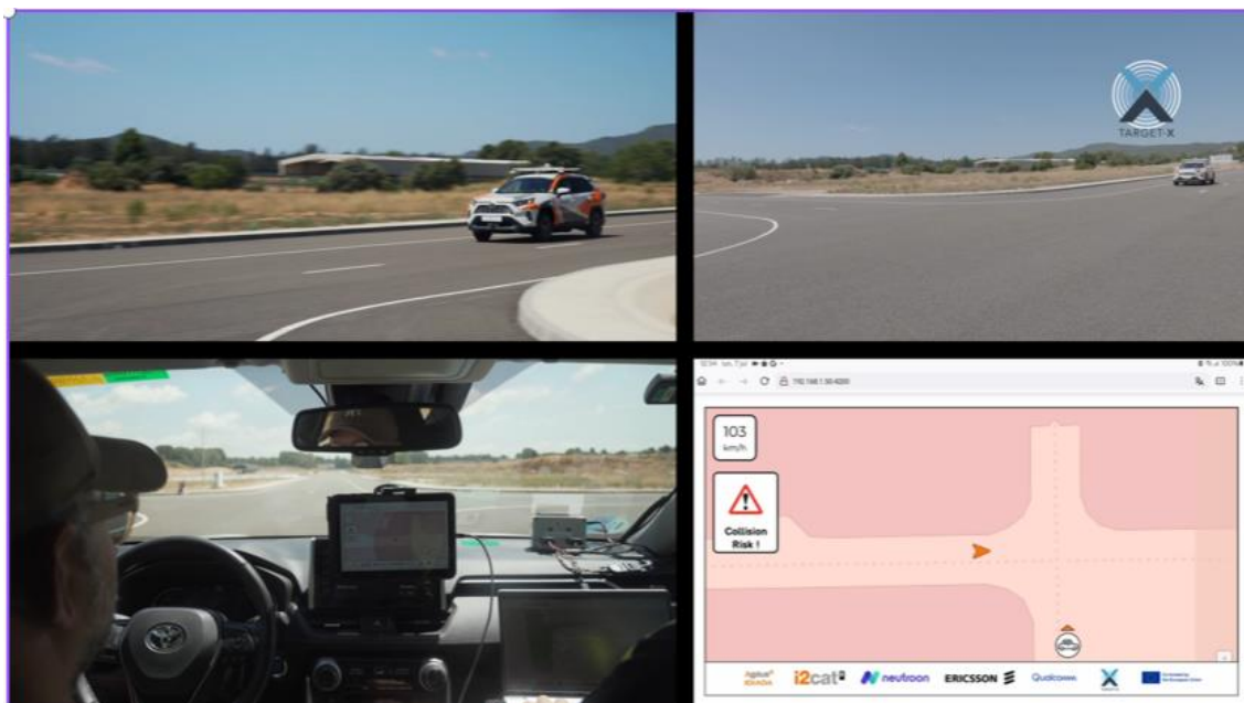
Figure 6.3 Snapshot of the digital twin showing vehicle-in-the loop.
