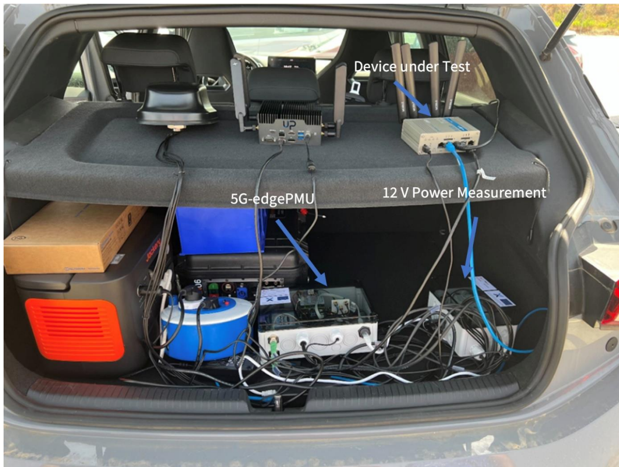
Figure 3.5 5G-edgePMU mounted in a car for power consumption measurement
