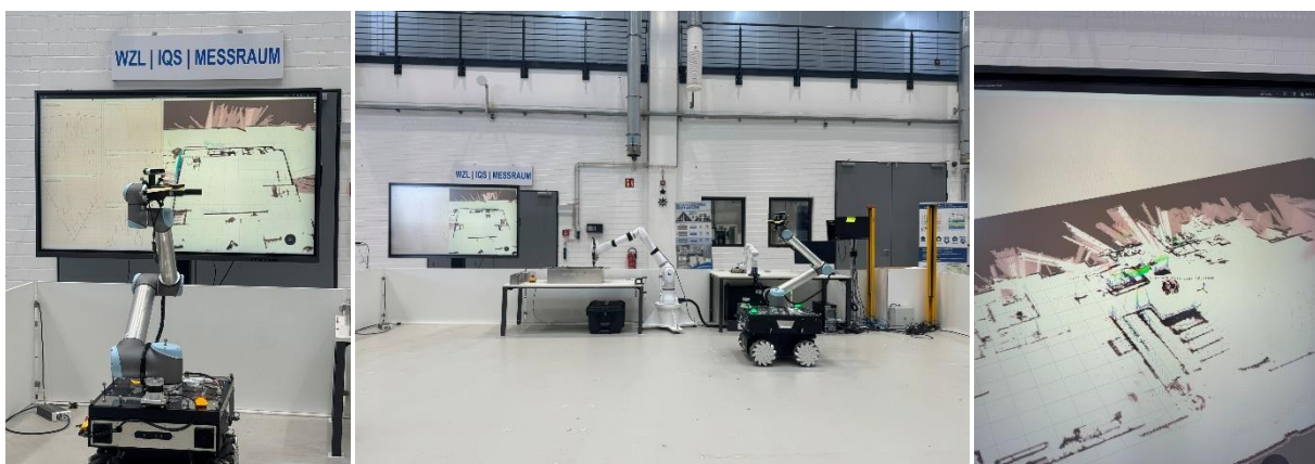
Figure 5.6 Photographs of the 5G-Based Positioning and LiDAR-SLAM trials conducted at the WZL Testbed. Source: from [TAR25-D2.5].
