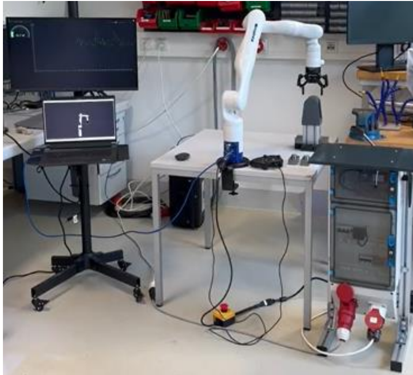
Figure 3.4 Kinova robot arm moving a fixture with variable weights and measured by the Meter-X device.
