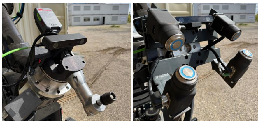
Figure 10: Final prototype of end effectors left the unbolting end effector, right the gripping end effector.
