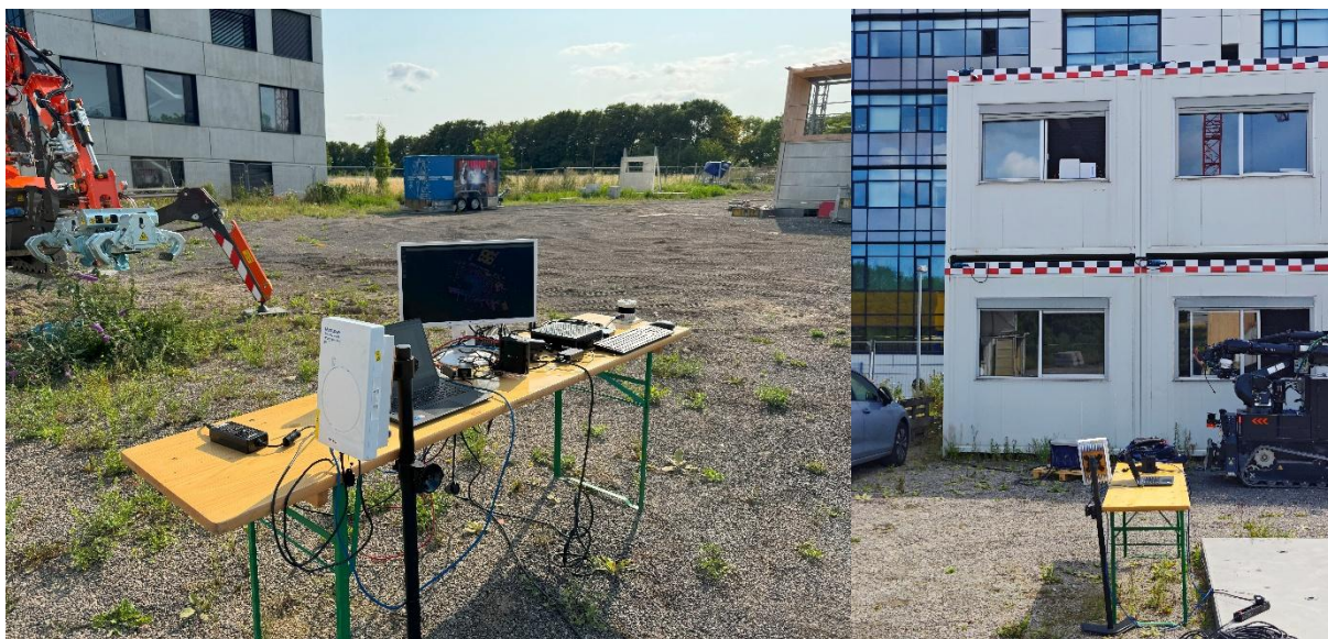
Figure 17: Qualcomm mmW Travel Kit test equipment and setup on the construction testbed
