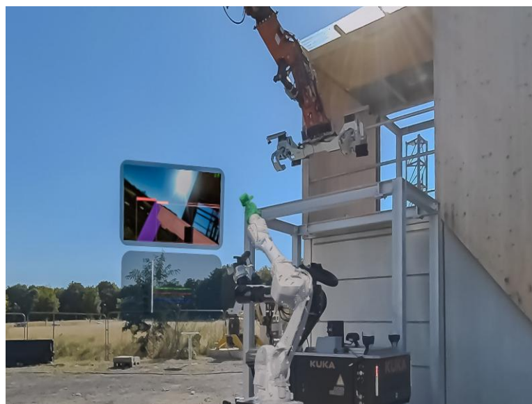
Figure 14: Simulation and control of the robot via XR.
