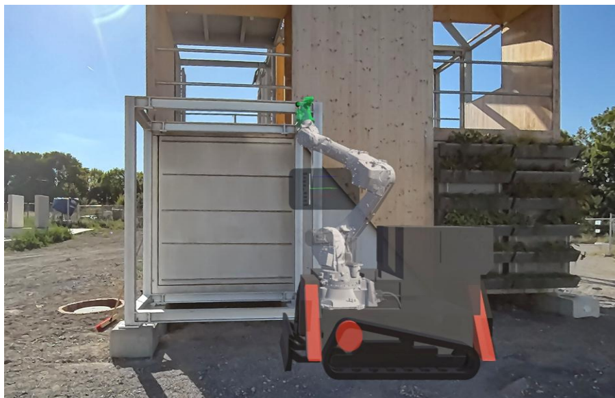
Figure 12: Reachability test using the HMD before deploying the machine.
