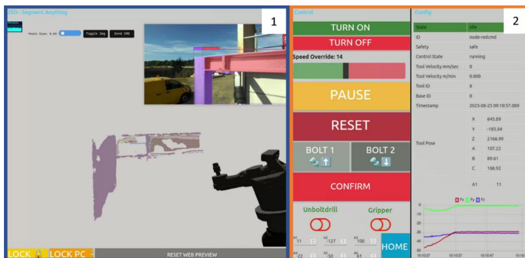
Figure 9: User interface for the monitoring of unbolting process, 1) bolt-finder UI, presents the interactable 3D environment with point cloud and robot as well as the segmented image. 2) meta-controller UI, presents the process commands buttons and live robot state and force/torque feedback.
