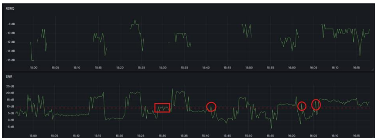
Figure 29: Time periods when the orchestrator is not triggers although the SNR is below 9 dB.
