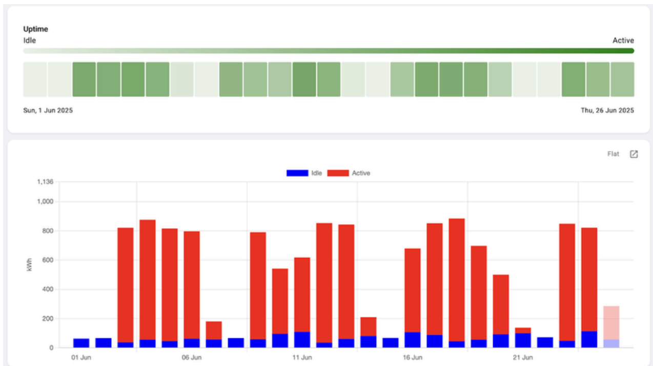
Figure 77: Energy data of industrial machine and analysis where working state is identified.
