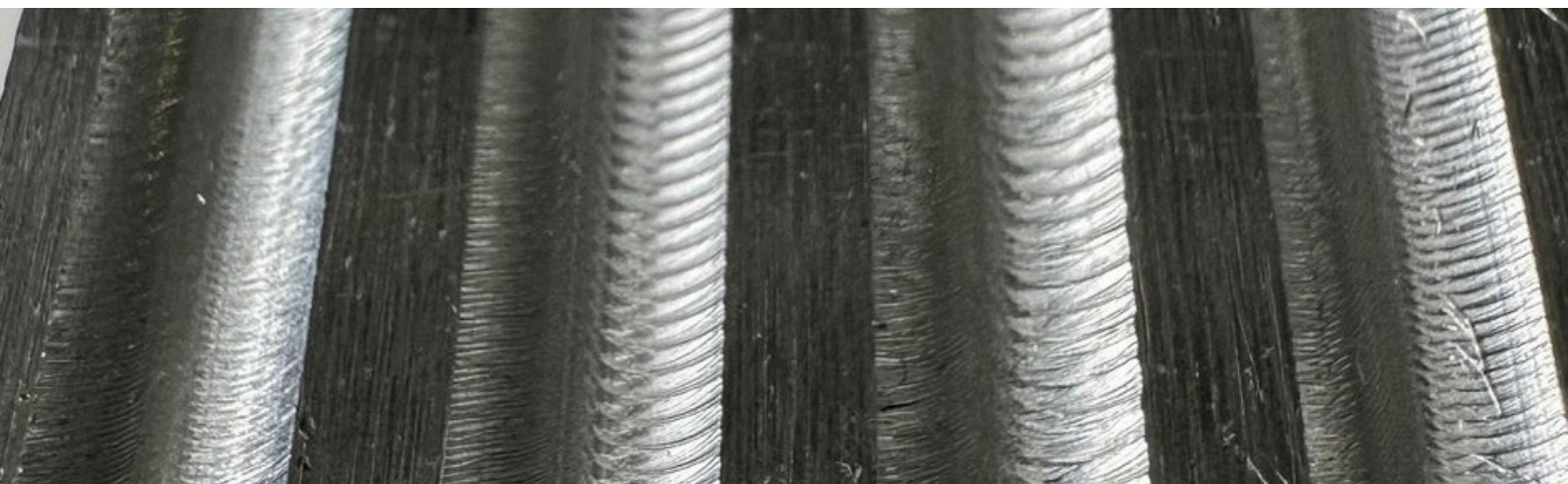
Figure 7: Surface of the workpiece with and without chatter.
