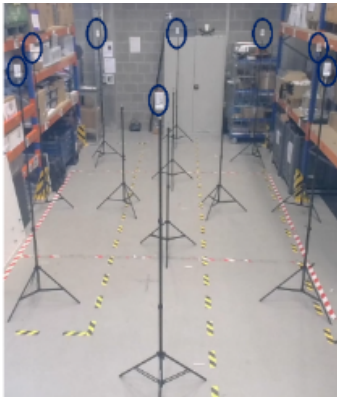
Figure 93: UWB setup and coverage
