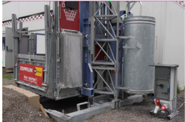
Figure 34: Mounted 5G edgePMU in electronics lab ACS-RWTH(left), Second design iteration of Meter-X connected to the material hoist on the construction testbed (right)
