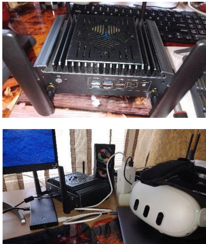
Figure 65: Test bench with 5G/WiFi edge device with OCULUS VR/XR glasses Connecting through public network to microservices server
