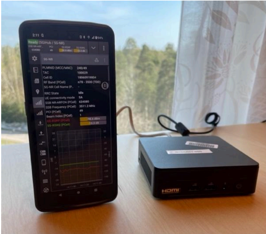
Figure 140: The portable setup of the INTERACT-B5G Project (Client: Crosscall device with Qualipoc; Server: ASUS NUC 12WSK).
