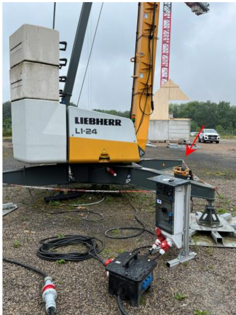
Figure 4-2: Meter-X connected to a Small Tower Crane
