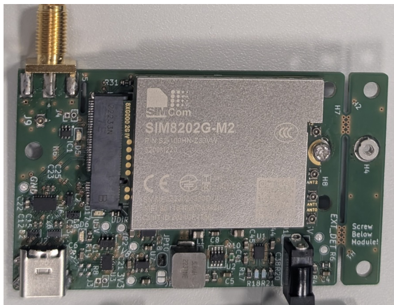
Figure 10: The assembled carrier board with module attached.
