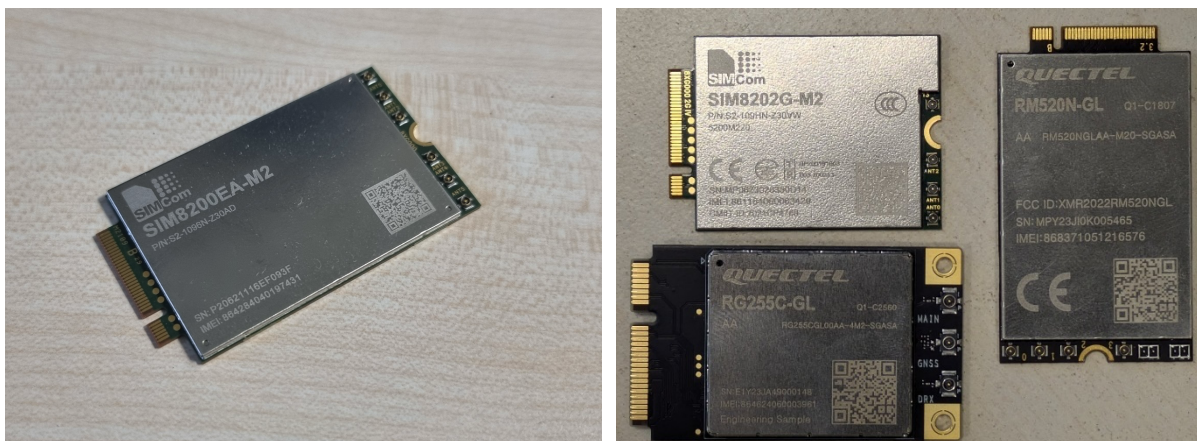
Figure 7: Different M2 module for 5G connectivity with onboard antenna connectors that are evaluated.
