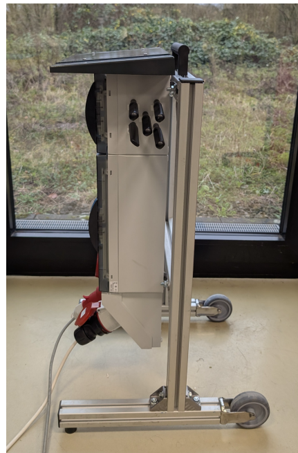
Figure 19: Measurement box for outdoor inline measurement of voltage current and energy, with adapters for one phase measurements.
