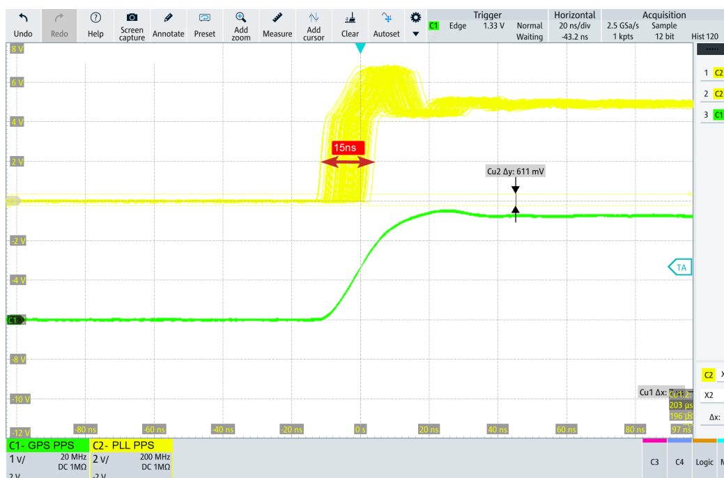
Figure 16: Jitter measurement of the PLL after compensation using a high quality oscillator. (Green: GPS PPS, Yellow: PLL PPS, 120 captures)
