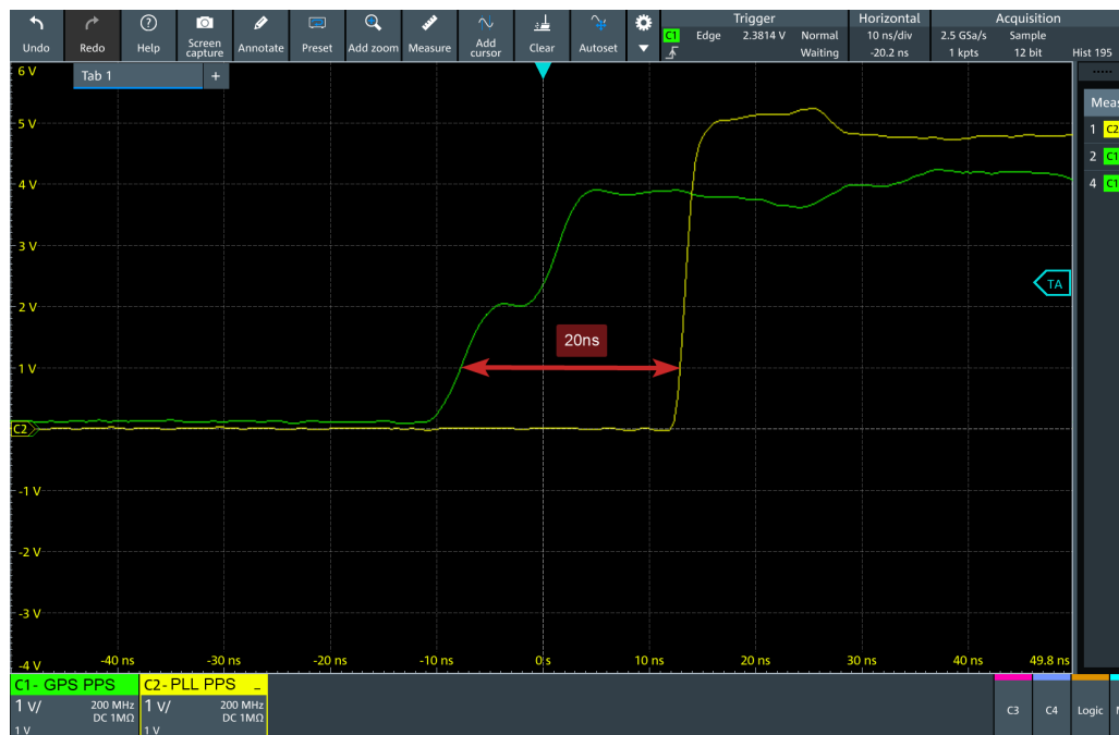
Figure 15: Performance measurement of generated PPS signal of the PLL. (Green: GPS PLL, Yellow: PLL PPS)
