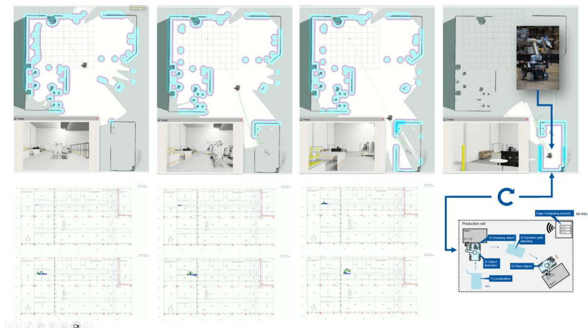
Figure 2.2: Overall layout of the use case, illustrating the robot's localization on the shop floor and the designated location for the pin-picking task. The bottom left section shows the benchmarking results of 5G positioning, displayed on the 5G dots map.
