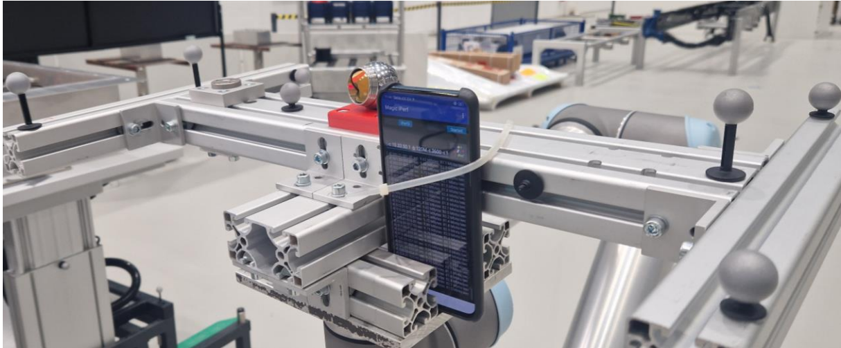
Figure 3.7: Initial trials on Benchmarking of Localization via 5G NR with a Mobile Manipulator at WZL Testbed.
