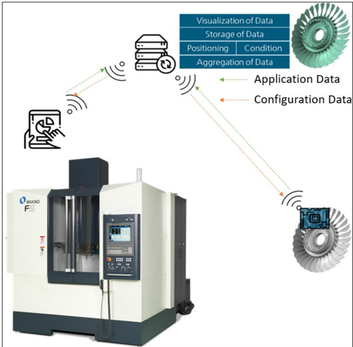
Figure 2-3: Systematic Architecture Diagram of the Track and Tracing of Workpieces Use Case [1]
