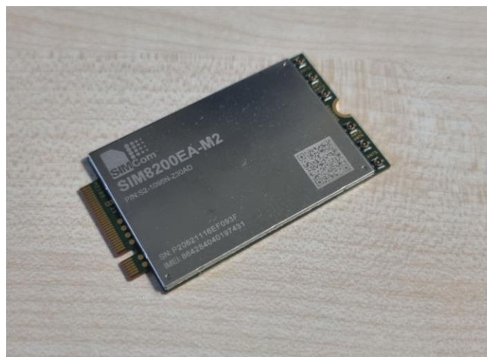
Figure 4: SimCom SIM8200EA-M2 module for 5G connectivity with onboard antenna connectors.
