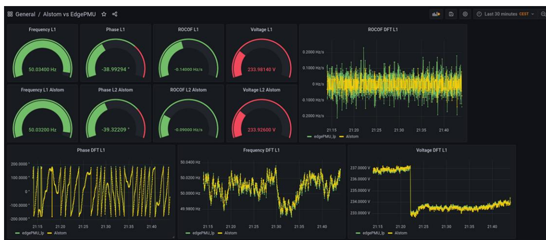
Figure 20: Example Grafana UI showing PMU measurements, currently with a manually configured interface.
