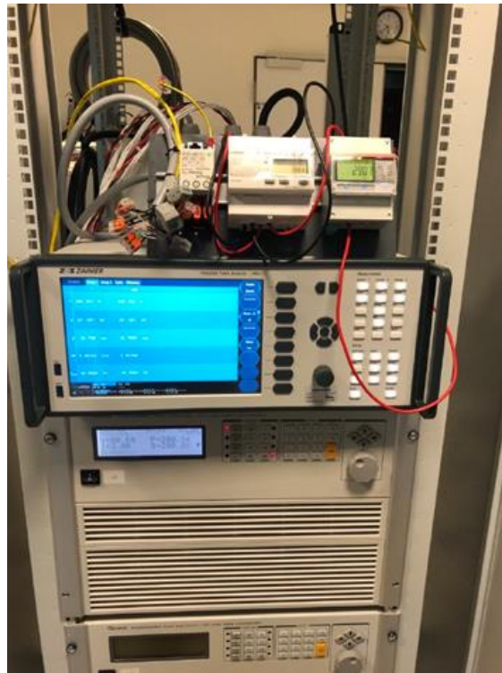
Figure 9: Energy meter validation with the two metering devices at the top, the Zimmer power analyzer in the middle and the Chroma AC/DC load on the bottom.
