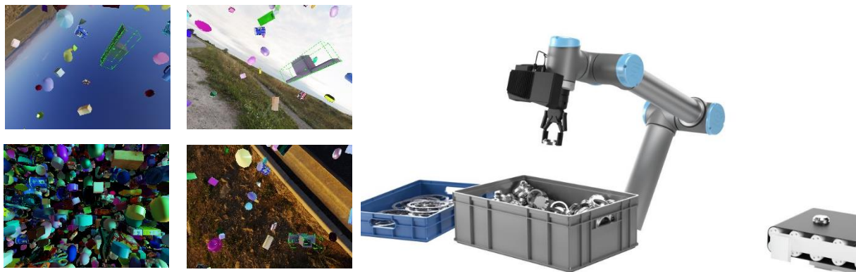
Figure 3.4: On the left is the generated synthetic data used for the training of the pose estimation algorithms for object detection [7]. On the right is the pick and place with object detection [12].
