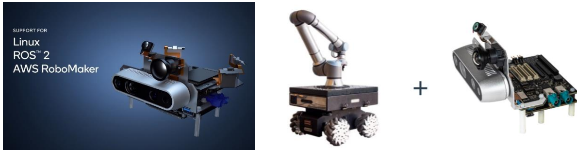
Figure 4.2: Qualcomm robotics kit RB5. Source: adapted from [15].
