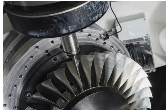
Figure 4: Milling of a BLISK with integrated 5G-Sensor for wireless monitoring of the workpiece.
