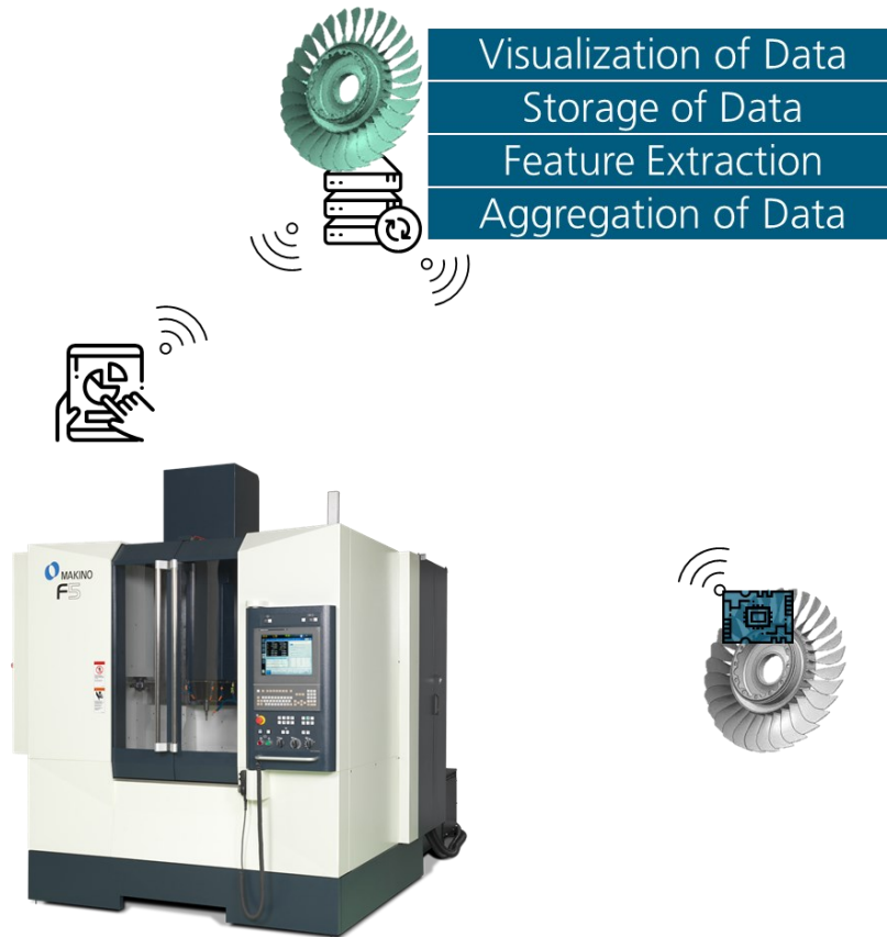
Figure 3 : Track and tracing of the assets using 5G wireless sensor platform.
