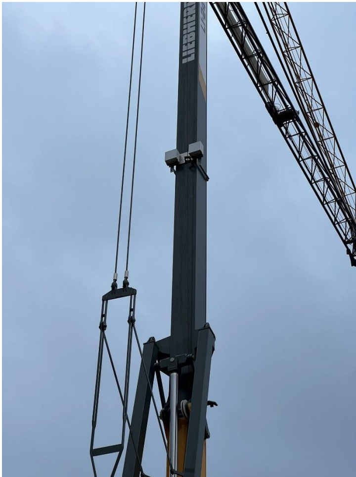
Figure 4.2 Tower crane converted to 5G antenna [18]
