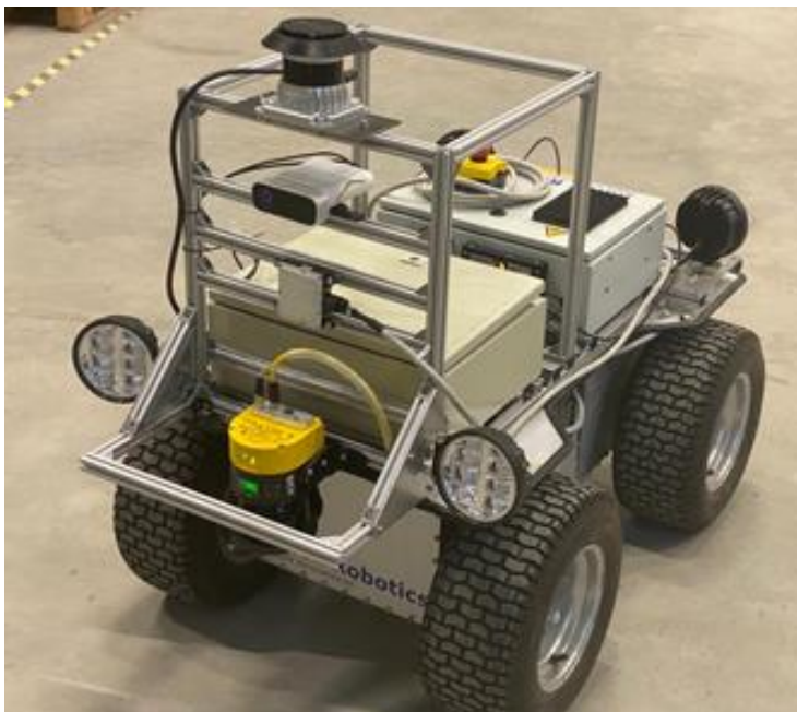
Figure 3.4 Four-wheel, mobile robot platform by Innok Robotics with additional equipment for environment capture.
