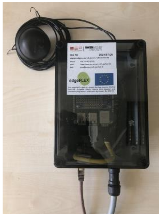
Figure 1: edgePMU with GPS and signal connection
